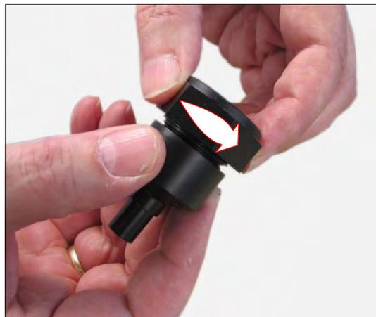
3. Clean the ball of the condensate drain valve or replace it, if required.
