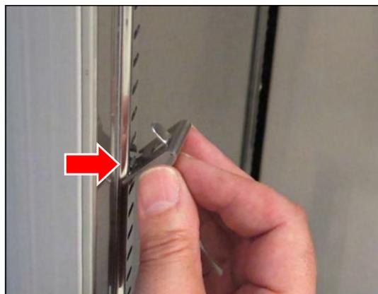
4. Press the mounting clip together from below and insert also the lower part into the fastening rail.
