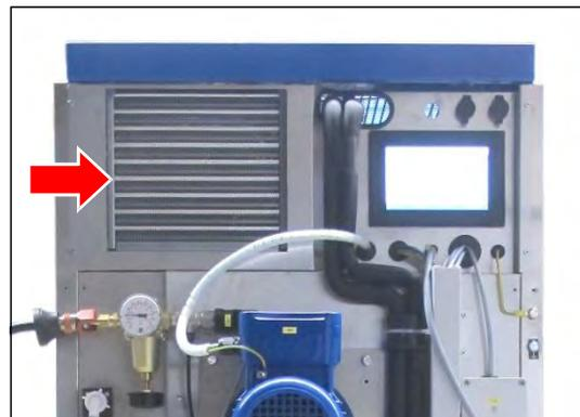
1. Aspirate the fan grill using a vacuum cleaner or clean it by hand using a smooth brush.
