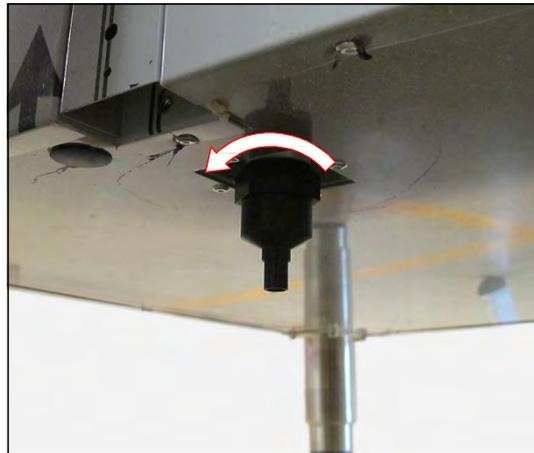
2. Unscrew the condensate drain valve.
