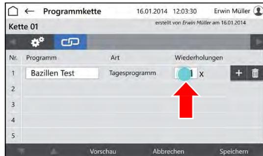
16. Touch the button INSERT ROW to insert a new program row and to add a further program to the program chain.
