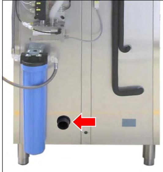
2. Connect a conductive vent hose and fasten it by means of a hose clamp. (External diameter of the connection: 60 mm).
